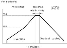
Iron Soldering times: 1 times max Fig.2
