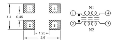
To be sure the consistency of the copper foil size under the PAD openings on both sides to prevent tombstone, solder empty and component shifted effect.
