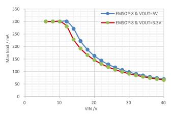
Figure 37. Maximum Output Current vs Input Voltage, eMSOP3x3-8,T<sub>J</sub> ≤ 150°C
