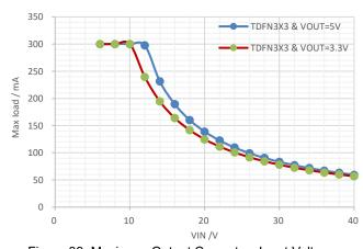
Figure 39. Maximum Output Current vs Input Voltage, TDFN3X3-8,TJ ≤ 150°C
