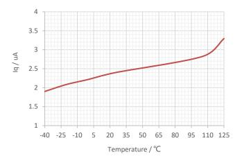
Figure 3. Quiescent Current vs Ambient Temperature
