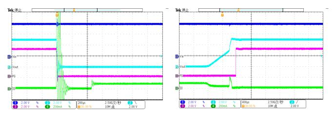
Figure 56. Enter Short Circuit Protection
