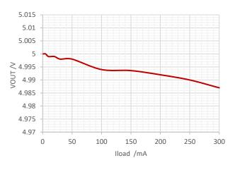
Figure 10. Output Voltage vs Output Current
