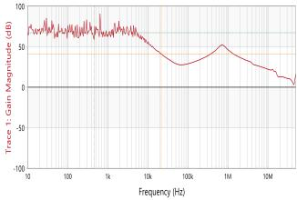
Figure 13. PSRR vs Frequency at lout=10mA, Cout=4.7uF
