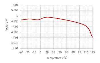
Figure 7. Output Voltage vs Ambient Temperature at VOUT=5V
