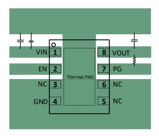
Figure 64. PCB Layout Example
