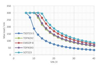
Figure 31. Maximum Output Current vs Input Voltage, VOUT=3.3V of Different Packages ,TJ ≤ TSD\_R
