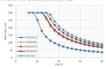
Figure 30. Maximum Output Current vs Input Voltage, VOUT=5V of Different Packages ,TJ ≤ TSD\_R
