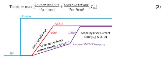
Figure 22. Soft-start Waveform vs Output Capacitor
