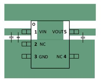
Figure 63. PCB Layout Example
