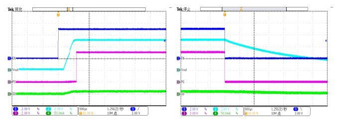
Figure 46. Enable (Iload=10mA)
