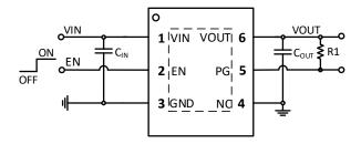
Figure 26. SCT71403Q Typical Application Schematic
