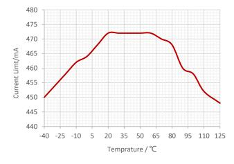
Figure 11. Output Current Limit vs Ambient Temperature
