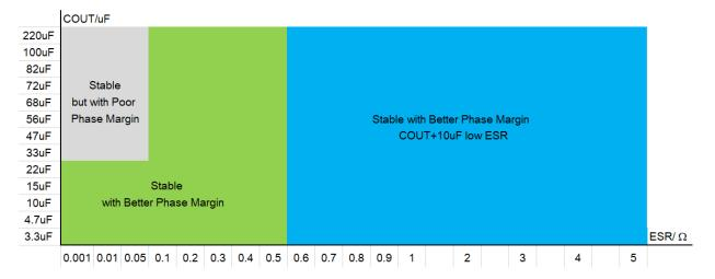
Figure 29. SCT71403Q Stability vs Output Capacitor
