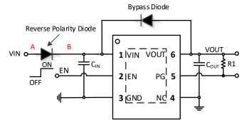
Figure 27. SCT71403Q Typical Application Schematic with Reverse Polarity Diode
