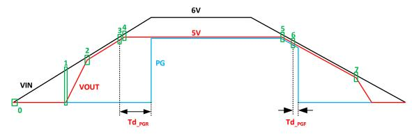
Figure 25. Startup and Shutdown Example —SCT71403Q Series
