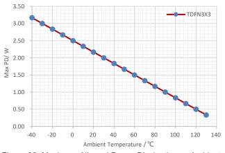
Figure 38. Maximum Allowed Power Dissipation vs Ambient Temperature, TDFN3X3-8,TJ ≤ 150°C
