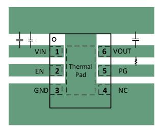
Figure 60. PCB Layout Example
