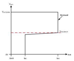
Figure 21. Current Limit with Foldback Feature
