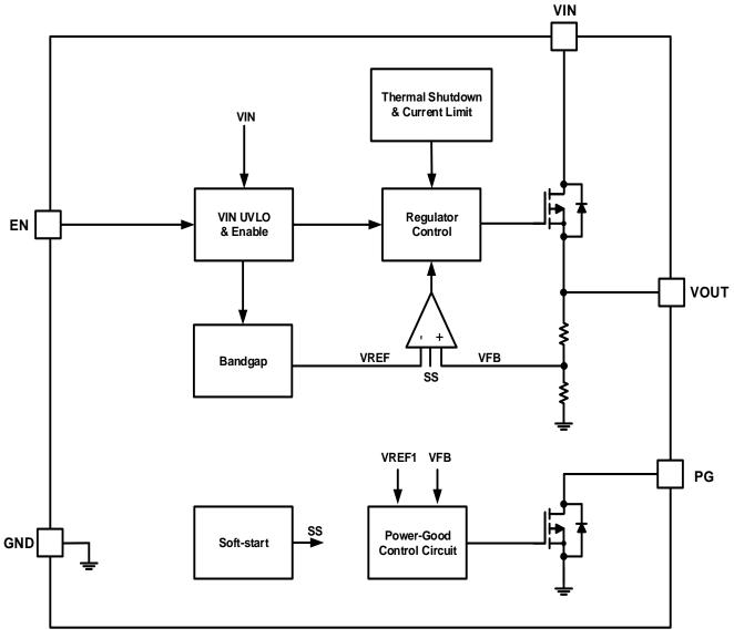
Figure 19. Functional Block Diagram
