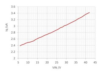
Figure 2. Quiescent Current vs Input Voltage, No load
