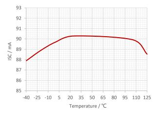
Figure 12. Short Current Limit vs Ambient Temperature
