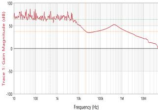
Figure 17. PSRR vs Frequency at lout=10mA, Cout=22uF
