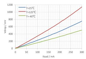
Figure 6. Dropout Voltage vs Output Current
