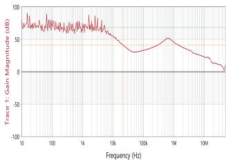
Figure 15. PSRR vs Frequency at lout=10mA, Cout=10uF
