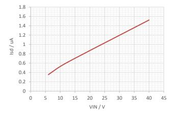
Figure 5. Shutdown Current vs Input Voltage
