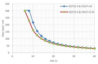
Figure 35. Maximum Output Current vs Input Voltage, SOT23-5,T<sub>J</sub> ≤ 150°C
