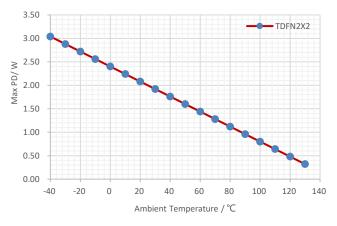
Figure 32. Maximum Allowed Power Dissipation vs Ambient Temperature, TDFN2X2,TJ ≤ 150°C
