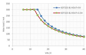
Figure 41. Maximum Output Current vs Input Voltage, SOT223-4,TJ ≤ 150°C
