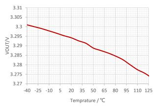
Figure 8. Output Voltage vs Ambient Temperature at VOUT=3.3V
