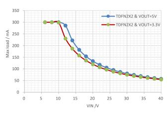
Figure 33. Maximum Output Current vs Input Voltage, TDFN2X2,TJ ≤ 150°C
