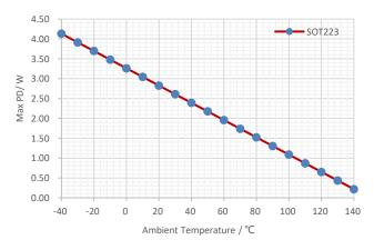
Figure 40. Maximum Allowed Power Dissipation vs Ambient Temperature, SOT223-4,TJ ≤ 150°C
