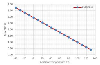
Figure 36. Maximum Allowed Power Dissipation vs Ambient Temperature, eMSOP3x3-8,TJ ≤ 150°C
