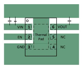
Figure 61. PCB Layout Example
