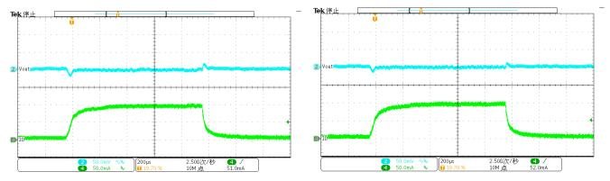
Figure 52. DC-DC Load Transient (1mA-100mA),VOUT=5V
