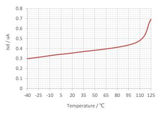
Figure 4. Shutdown Current vs Ambient Temperature
