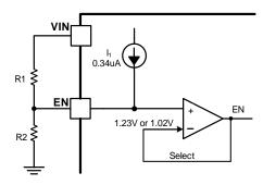
Figure 20. System UVLO by enable divide
