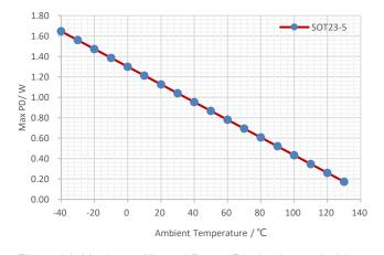
Figure 34. Maximum Allowed Power Dissipation vs Ambient Temperature, SOT23-5,TJ ≤ 150°C
